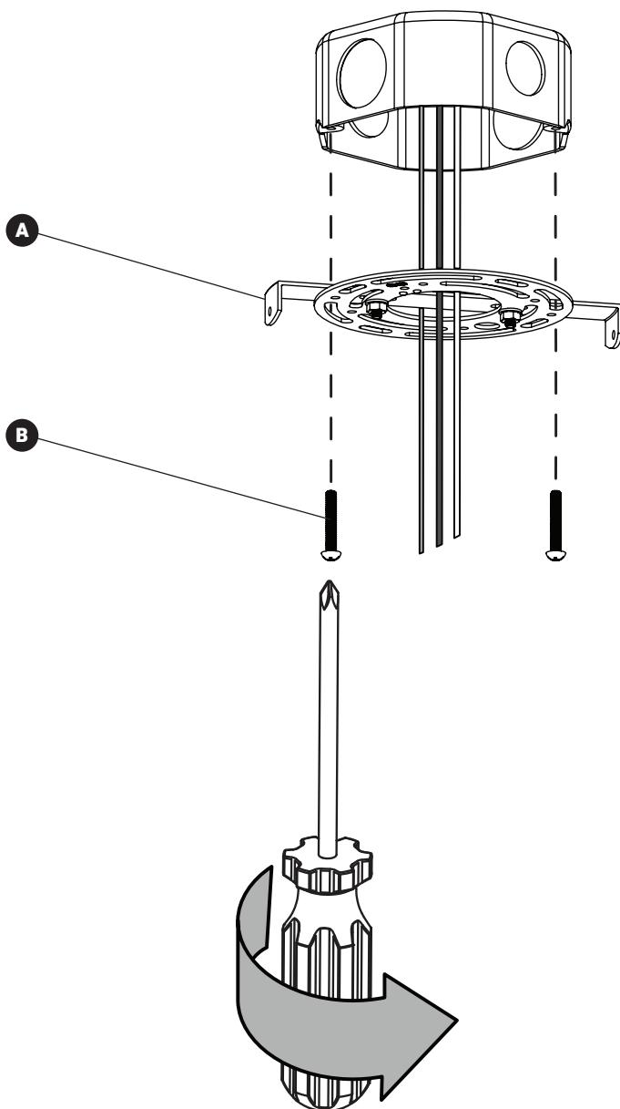
**4** CONNECTING THE WIRES AND INSTALLATION OF THE CANOPY
